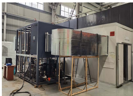
图 2 低温干燥冷藏调湿多功能储粮设备实验台 Fig.2 Experimental bench of multi-functional grain storage equipment for low temperature drying, refrigeration and humidification
