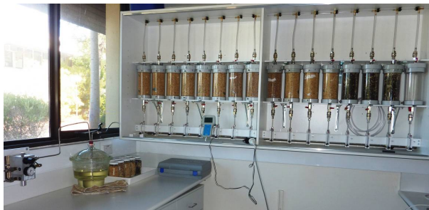
Fig.1 A gas purging flow system was used to treat the insects with constant concentrations of nitrogen and oxygen and maintained low carbon dioxide concentrations during the period of treatment. All 15 cylinders were filled with a known amount (1.8~2 kg) of grain (wheat, barley, oats, lupin and canola). A sealed sachet made of muslin cloth with 40~50 g of mixed age culture of stored grain insects with >200 adults were inserted at a depth of 6 and 23 cm.
