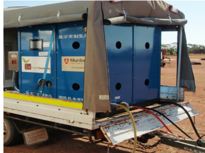
Fig.3 Nitrogen is produced via 60 m 3 /hr, 99% purity Membrane separation Nitrogen Generator. Hose of diameter 3/4" connected to outlet.
