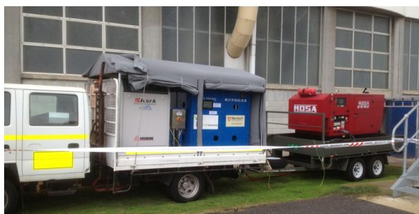
Fig.1 Mobile fumigation unit comprising compressor, membrane separation nitrogen generator and diesel generator outside grain storage at the Kwinana terminal.
