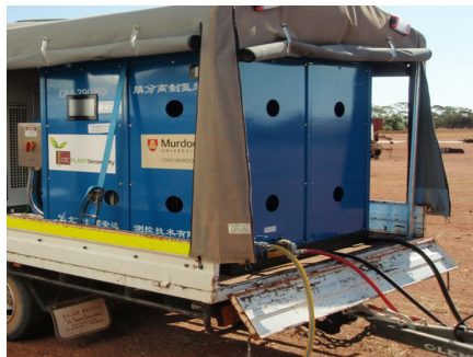
图 3 通过 60 m 3 /h、99% 纯度的膜分离制氮机生产氮气, 直径为 3/4 英寸的软管连接到出口。 Fig.3 Nitrogen is produced via 60m 3 /hr, 99% purity Membrane separation Nitrogen Generator. Hose of diameter 3/4" connected to outlet.
