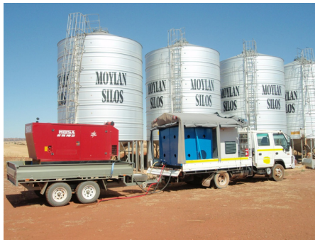
图 2 正在向 75 t 筒仓充入氮气。该膜分离制氮装置 (60 m 3 /h, 99% 纯氮) 可完全移动, 由柴油发电机提供动力。 Fig.2 Nitrogen application underway to 75 tonne silos. This Membrane Nitrogen generation unit (60 m 3 /hour, 99% pure nitrogen) is completely mobile being powered by a diesel generator.
