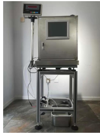
图 2 农产品干燥能源循环节能工艺智能实验系统 Fig.2 Intelligent test system for energy recycling and saving technology of agriculture products drying
